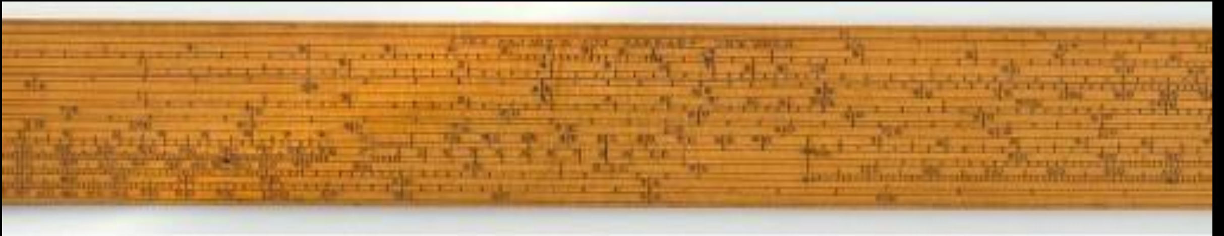
Example of a Typical 19 th Century 20 Inch Gunter Scale with Gunter's Initial Scales and Numerous Other Additional Scales Later Proven Useful in Navigation
