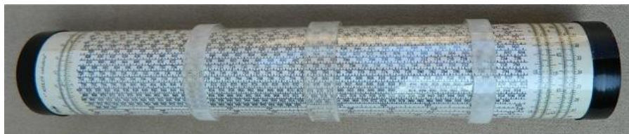
Muto Giken Kooler Calculator cylindrical slide rule. Sold for $700. This is a rare Japanese cylindrical slide rule with a 490 cm length scale in 50 sections. Made sometime after WWII. I have seen one other example of this slide rule. Photo from eBay
