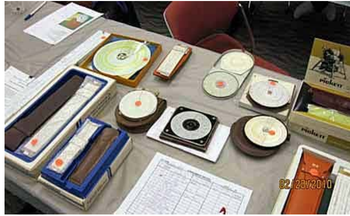
Another collection of circular and standard slide rules.
