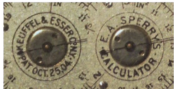
Figure 17. Details of Markings for Type 3b
