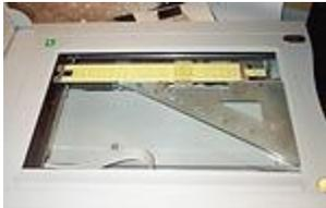
Demonstration of Michael O'Leary's slide scanning technique, with a Pickett rule positioned on an older model HP 4P scanner, using a glued-up set of drafting triangles.
